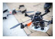
Career Academy. This device connects all of the other components of the drone such as the motors and battery. The Pixhawk also works as the gyroscope and accelerometer. He will also be learning and utilizing some of the same software that is used at the UNL drone labs.
